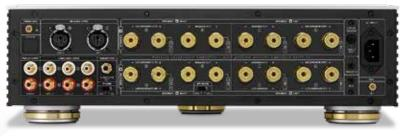
**ABOVE:** The one balanced XLR/three RCA line inputs are joined by an MM/MC phono input, subwoofer output and no fewer than 16x 4mm speaker cable posts. There are both A and B speaker banks with two amplifiers per 'channel' (one with optional high-pass filter) for either bi-amping or bridging into two, single channel amps
